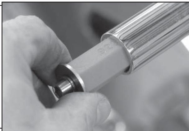
**STEP 1A - NOTE:** Not all handlebars are constructed from tubing that has the same inside diameter. For example, OEM Harley-Davidson handlebars use thin-wall stainless steel tubing. If your motorcycle does **NOT** have OEM Harley-Davidson handlebars made of thin-wall stainless steel tubing, proceed to **Step 2**.
