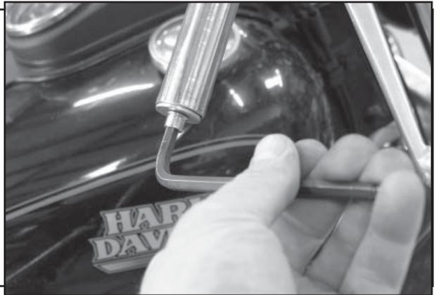
**STEP 3:** There is a small ball bearing pressed into the end of the throttle grip. Slide the throttle grip over the handlebar end until the bearing registers onto the bearing mount bolt as shown. Install the throttle cables onto the Battistinis grips as per the procedure outlined in the appropriate service manual for your year and model of motorcycle. Check for proper throttle operation before riding your motorcycle.
