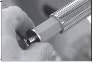
**STEP 1A - NOTE:** Not all handlebars are constructed from tubing that has the same inside diameter. For example, OEM Harley-Davidson handlebars use thin-wall stainless steel tubing. If your motorcycle does **NOT** have OEM Harley-Davidson handlebars made of thin-wall stainless steel tubing, proceed to **Step 2**.
