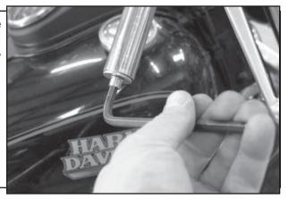
**STEP 3:** There is a small ball bearing pressed into the end of the throttle grip. Slide the throttle grip over the handlebar end until the bearing registers onto the bearing mount bolt as shown. Install the throttle cables onto the Battistinis grips as per the procedure outlined in the appropriate service manual for your year and model of motorcycle. Check for proper throttle operation before riding your motorcycle.
