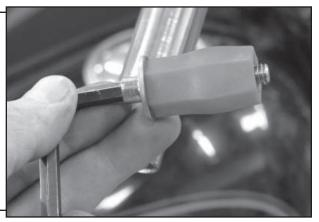
**STEP 2:** The large stainless steel washer will stop against the bar end when the insert is fully installed. As shown, tighten the bearing mount bolt. Avoid over-tightening this bolt so as not to damage the polymer insert.
