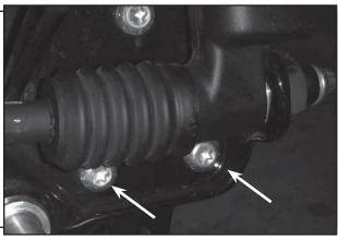
**STEP 2 - FOR 2008-UP MODELS:** Should the alignment between the master cylinder pushrod need adjustment, use the <sup>5</sup>/<sub>16</sub>" shim washers included with this kit. They are placed over the mounting screws (arrows) in between the master cylinder and the bracket. This will provide adjustment to allow for proper alignment of the brake arm with the master cylinder pushrod. This may not be necessary on every motorcycle.
