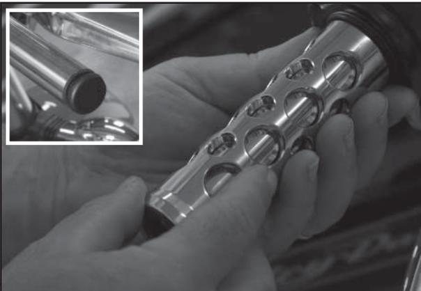
**STEP 2:** Now install the left-side grip. Remove the existing grip and clean the handlebar end if necessary. The new left-side grip is held in place with three stainless steel set screws. Use a drop of blue Loctite 242 on either the set screw threads or in each of the threaded holes in the grip. Slide the grip up the handlebar and position it to your preference. Tighten each of the three set screws a little at a time to ensure that they are all tightened uniformly, as shown.
