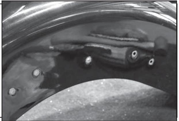
**STEP 5:** Use a drop of blue Loctite 242 on the threads of the 10-24 button head cap screws and install them using one internal star lock washer and one large diameter washer each. Start all 5 bolts and then tighten them all equally to ensure proper fit.
