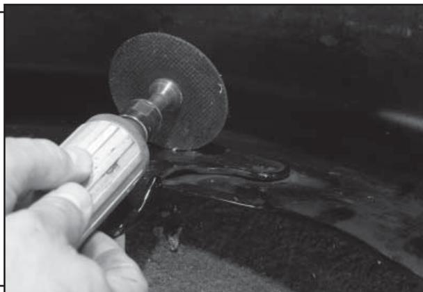
**STEP 2:** Prior to popping out the rivets, cut along their circumference on the outside of the fender. This prevents tearing or chipping the paint when they are removed.
